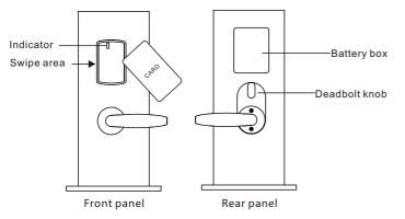
3-2: Lock from inside: Rotate the deadbolt knob on the rear panel for the double lock function (Note: The card needs to be encoded by the compatible management software and card encoder before use.
