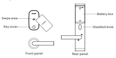
3-2: Lock from inside: Rotate the deadbolt knob on the rear panel for the double lock function (Note: The card needs to be encoded by the compatible management software and card encoder before use.
