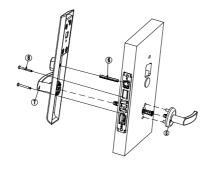
6: Align the hole position on the door panel and install the front sensing mask, insert the battery box on the rear panel and lock it with a long rod screw, install the battery, buckle the rear cover and lock it with a screw.
