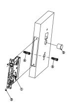
4: Fasten the front and rear panels with screws. Note that the holes in both panels should be aligned
