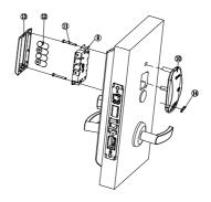
7: Install the strike plate and side plate
