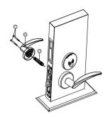
7: Insert the battery, install the battery box and side trim panel
