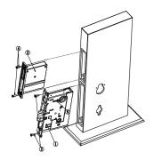
4: Install the Cylinder and front panel base and lock them with corresponding screws, Install front panel and Sensing panel,Lock the Cylinder as (6).
