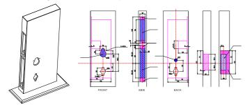
3: Install the lock body and battary box, Lock with screws.
