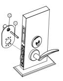
6: Install the rear panel handle assembly and lock it with long screws
